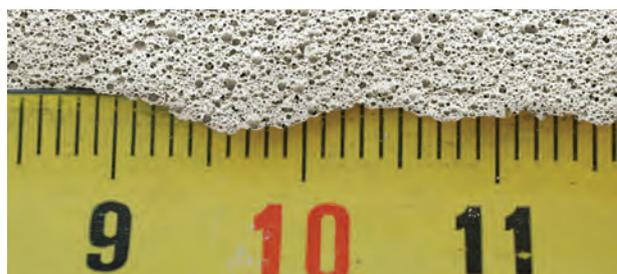
Terefil® is an engineered lightweight fill with a uniformly distributed cell structure.
