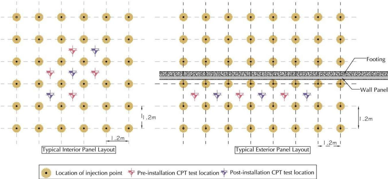
**Figure 1 - Typical Test Panel Layouts (Plan View)**
