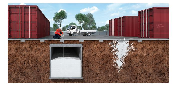
We inject one of our engineered structural resins beneath (or into) the construction of concern, filling any voids encountered to re-establish ground support. The Teretek® void-fill method may also be used for arresting water movement, and filling abandoned utilities and other man-made voids.
